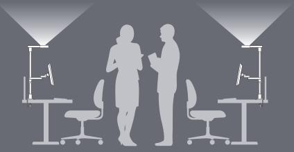
Uplights connect to room controls and provide glare-free, indirect ambient light for collaboration and general office tasks.
