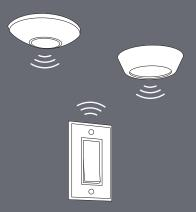
Sensors, room switches, and dimmers install without wires and operate without batteries.
