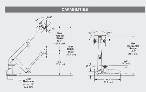
$<sup>^{\</sup>star}$  Joint is capable of rotating 360 degrees, but size of monitor will limit the rotation.
